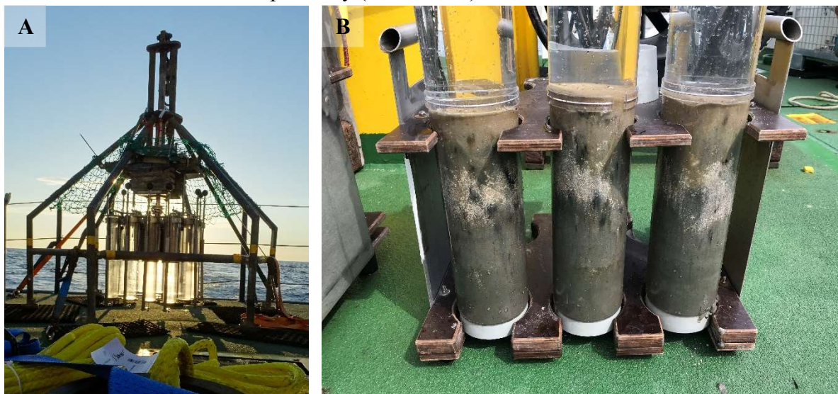
Fig. 5.8.1 A: Multicorer (MUC) prior to deployment on board, B: Three MUC cores containing benthos samples (photos: Sven Hoffmann).
