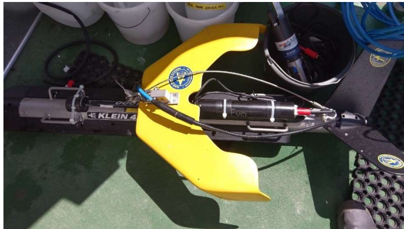
Figure 5.1.3 Sidescan system with mounted USBL positioning system
