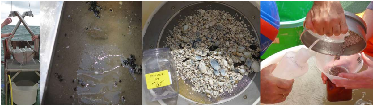
Figure 5.9.1 Photos illustrating sampling procedure. The two right-most photos show the fractions left on the 1.0 mm and 0.5 mm sieves.
