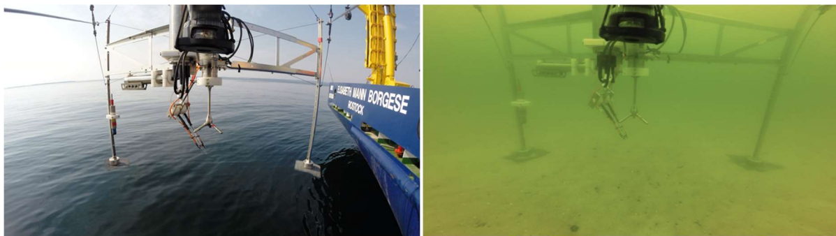
Figure 5.4.1 The EC lander during deployment (left) and at the seafloor (right) of the Oder Bank at 15 m depth.
