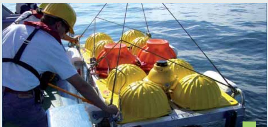
BATRE: DER INJEKTIONSSCHLITTEN WIRD ZU WASSER GELASSEN. / LAUNCHING OTIS – THE OCEAN TRACER INJECTION SYSTEM (FOTO: T. TANHUA / IFM GEOMAR)
