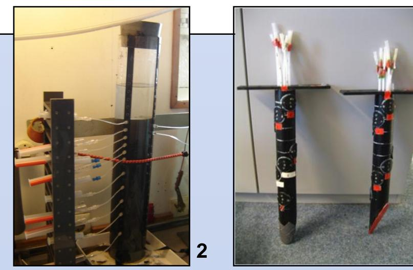
**Fig. 2 and 3: Pore water sampling** via rhizons (2) and groundwater lances (3).
