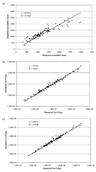
Fig. 5. A multiannual fit of simulated and measured data for the validation period (1990–1994): (a) streamflow, (b) Tot-N, and (c) Tot-P.
