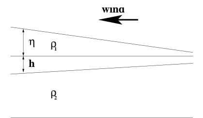
Figure 4.2. The wind induced surface elevation and the thermocline elevation.
