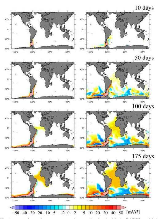
Fig. 8.22 Aspects of oceanic wave propagation, as simulated with the BARBI model (see Ap pendix B.2). The wave is initiated in Drake Passage by a baroclinic perturbation and propagates in the ocean wave guide around the globe. Left without topography, right with realistic topography Both simulations are for a mean state with prescribed Brunt–Väisälä frequency without any mean flow
