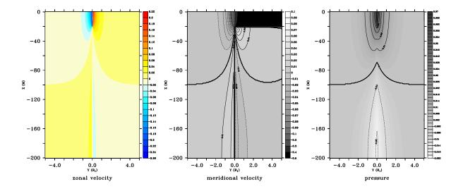
Figure 2.12. Zonal and meridional velocity and pressure perturbation near a wind edge. Pressure and zonal velocity are shown for t = 1/f. The mixing depth is 20 m, the baroclinic Rossby radius is about 6.4 km.
