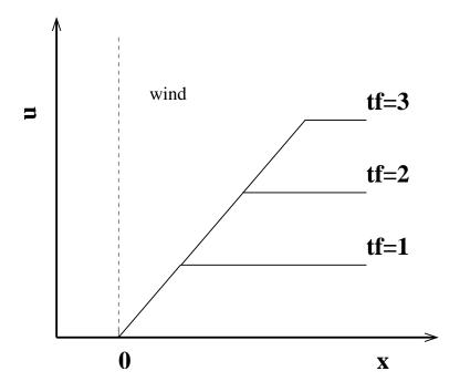
Figure 2.25. Kelvin waves arresting the coastal jet. Distant from the origin, the jet accelerates linearly with time and is independent of the coordinate x. When a wave front has passed through, u remains constant with time. The value depends on the time of arrest and is growing linearly with the distance of the origin.
