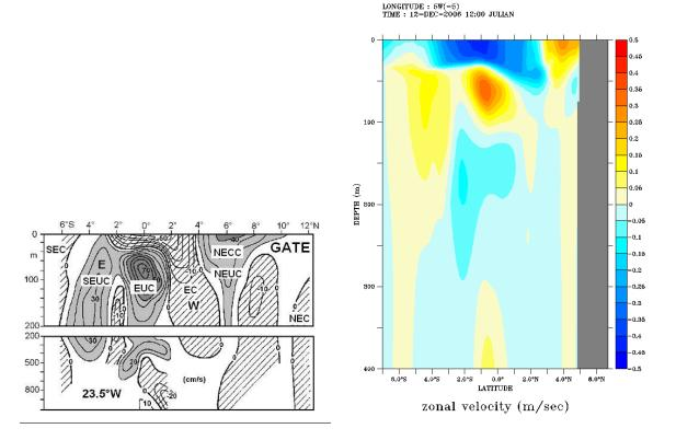
Figure 4.1. The equatorial currents found during the GATE experiment in the 60th (left) and seen in a numerical simulation (right).
