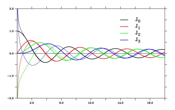
Figure C.1. Bessel functions of the first kind. Thick lines mark the full soltion, thin lines the asymptotic approximation.
