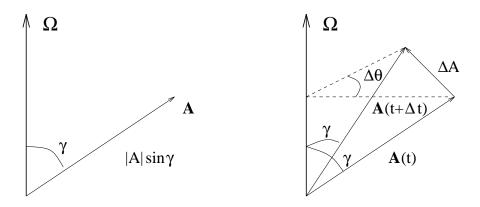
Figure 2.5. Rotation of a vector **A** with an angular velocity  $\Omega$ .
