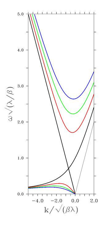
Figure 5.14. The dispersion relation of the equatorial waves spectrum. thin black: m = -1, thick black: m = 0, red: m = 1, green: m = 2,
