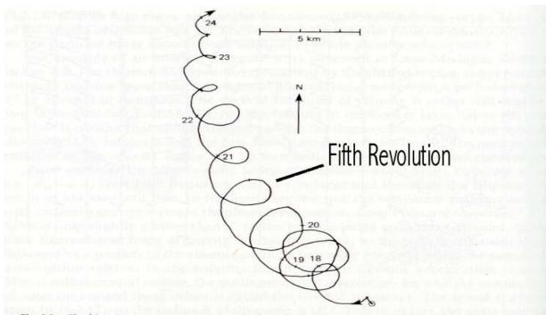
Fig. 8.3. The historic current measurements in the Baltic by Gustafson and Kullenberg (1936), showing oscillations of near-inertial period. The plot is a progressive vector diagram, showing the displacement a particle would have, given the velocity observed at the current meter.
