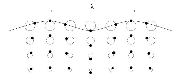
Figure 4.1. Orbital movement of fluid elements in relation to a monochromatic surface gravity wave.
