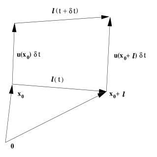
Figure 2.1. Deformation and rotation of a length vector **l**. The fluid element at  $\mathbf{x}_0$  moves with a different velocity than that at  $\mathbf{x}_0 + \mathbf{l}$ . After time  $\delta t$  the vector appear stretched and rotated.
