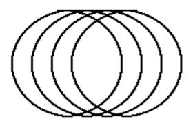
Figure 4.3. Spiraling orbital movement of fluid elements with consideration of the Stokes drift.
