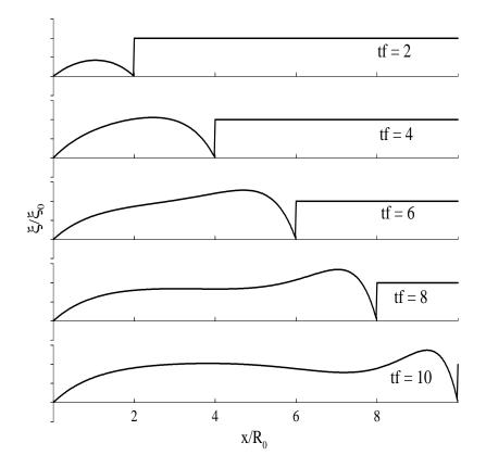
Figure 5.3. Sea level response to an initial step-like elevation at x = 0
