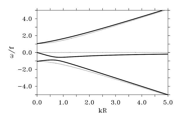
Figure 5.9. The dispersion relation of free waves in the open ocean. The nearly parabolic branches correspond to Poincaré waves, the other branch to Rossby waves. The dashed lines depict the f-plane approximation.
