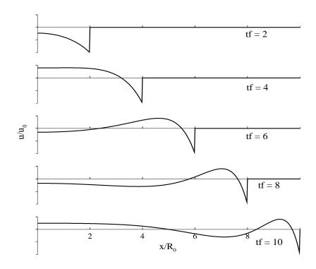
Figure 5.4. *u*-componente in response to an initial step-like elevation at x = 0
