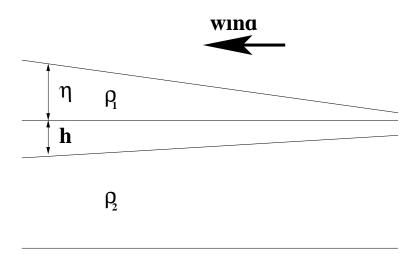
Figure 5.13. The wind induced surface elevation and the thermocline elevation.
