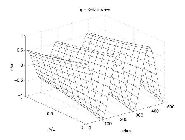
Figure 5.7. The undulating sea level for Kelvin waves. Note, the x- and y- coordinates are exchanged compared with the text. (Figure by W. Fennel)
