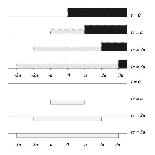
Figure 4.9. The spreading of waves in resonse to an initial step-like elevation, upper: sea level, lower: velocity
