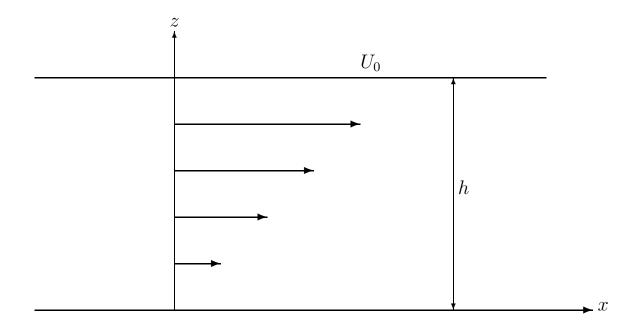
Figure 2.4. Velocity profile from friction within a Newtonian fluid.
