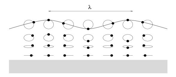
Figure 4.2. Orbital movement of fluid elements in relation to a monochromatic surface gravity wave for finite depth.
