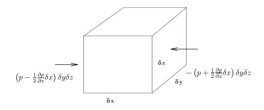
Figure 2.6. Effective pressure force on a volume element from a pressure gradient
