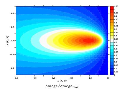
Figure 5.10. The frequency, scaled with the maximum frequency in dependency on the wave numbers.
