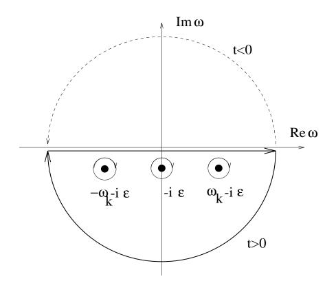
Figure 5.2. Integration path in the complex  $\omega$ -plane. For t < 0 there are no poles enclosed in the upper half-plane, for t > 0 all poles in the lower half-plane are enclosed by the integration path.
