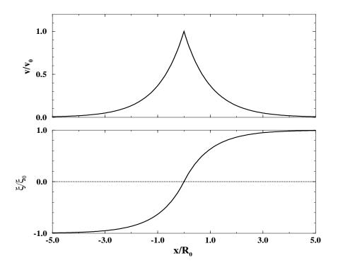
Figure 5.1. Geostrophic currents and sea level elevation as final state developing from a initial step like perturbation.
