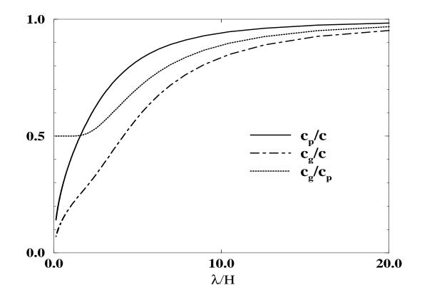
Figure 4.4. Phase and group velocity of surface gravity waves as function of the wave length. The ratio to the shallow water approximation  $c_p = c_g = c = \sqrt{gH}$  is shown.
