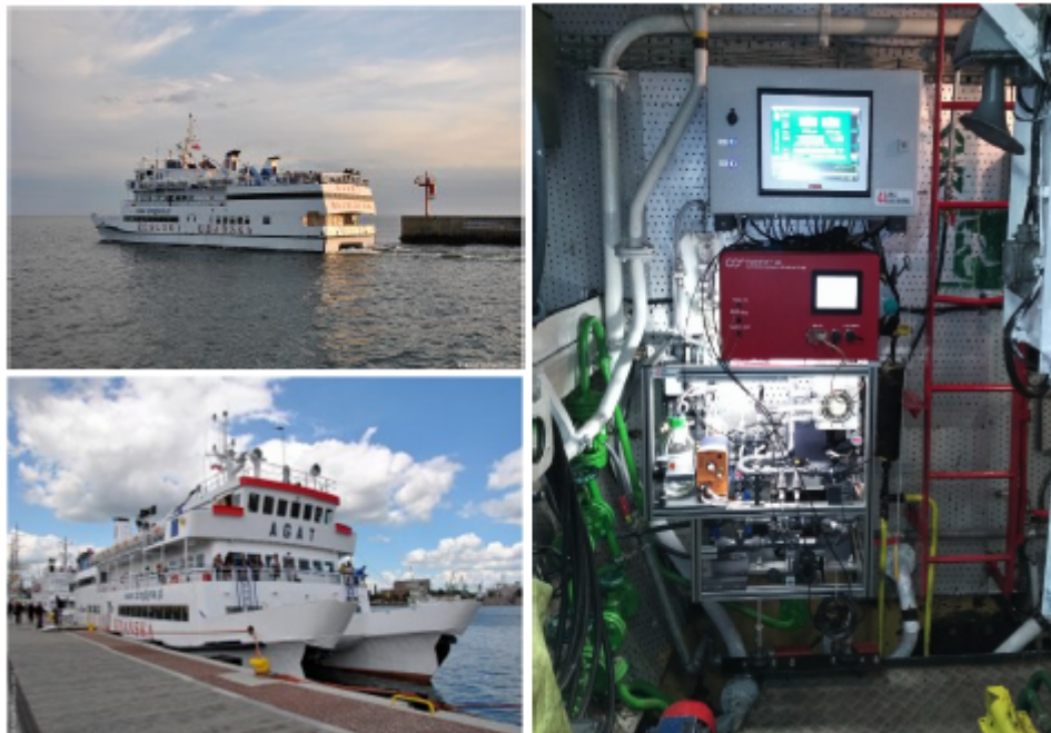
Figure 7. Ferrybox system (right) installed on VOS Agat (left).
