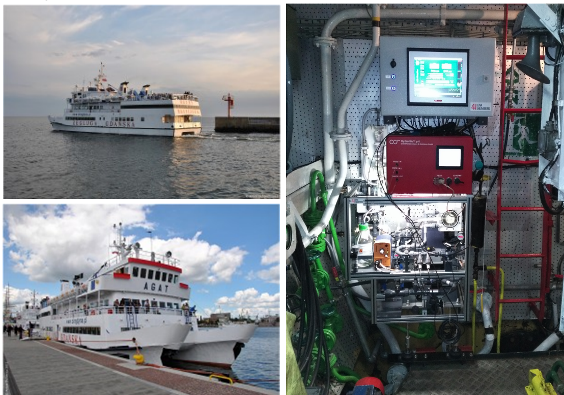
Figure 5: Upper and Lower Left - SOOP Agat (source: www.naszbaltyk.com ), Right - ferrybox installed in the engine room of the vessel.
